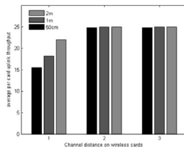
Fig. 3. Average per interface udp throughput for two 802.11a sending udp traffic to two different clients. The two links are tuned at adjacent channels 100 and 104. Physical interface separation is indicated by the color-code of the bars.
