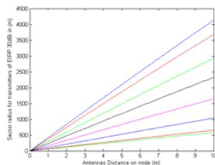
Fig. 1. The scenario assumes a mesh node of 2 back-to-back 802.11a interfaces, tuned to adjacent channels, with 180°, 13dBi gain and 20dB f/b antennas, spaced apart as indicated on the x-axis. The Y-axis is the maximum distance for successful reception of a 30dBm EIRP 802.11a client transmitting to one of the interfaces of the mesh node, while the other mesh interface is transmitting at 17dBm. Bottom-up on the plot are the curves for rates of 54, 48, 36, 24, 18, 12, 9 and 6Mbps.
